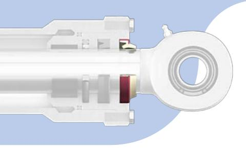
Hydraulic cylinders operate in a variety of applications and environmental conditions, including exposure to dust, debris or outside weather conditions. To prevent these contaminants from entering the cylinder assembly and hydraulic system, wiper seals (also known as scrapers, excluders or dust seals) are fitted on the external side of the cylinder head.
